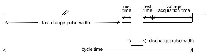
Figure 4: Charge cycle showing charge and discharge current pulses
