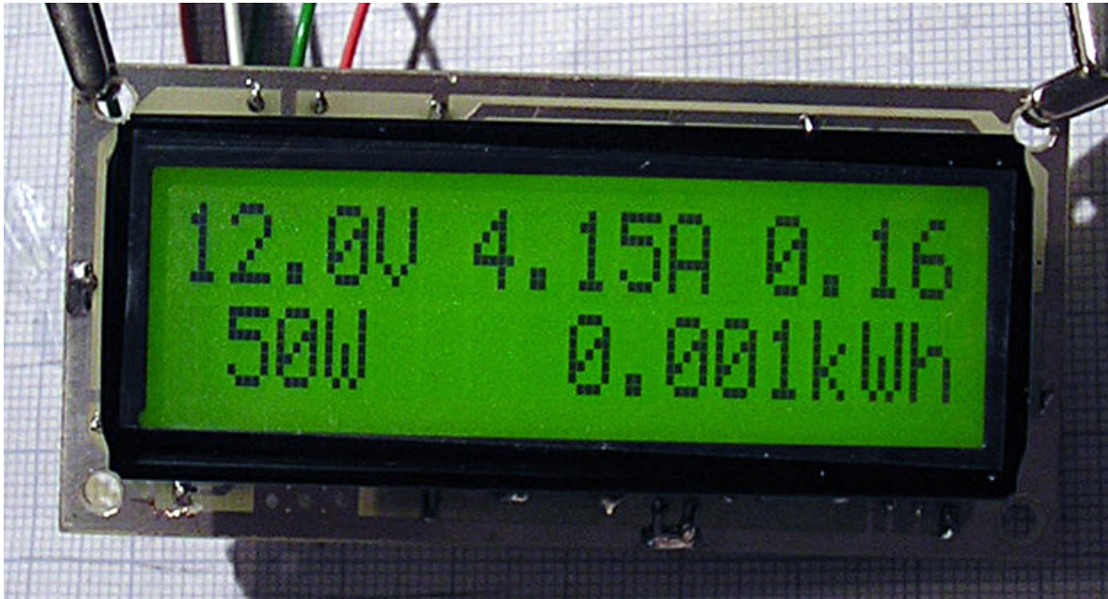
LCD-display with 2x16 character-Version
